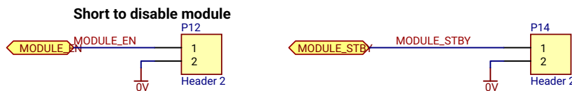
Figure 14 Module enable & standby headers
